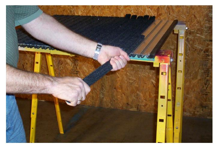
NOTE: Removal of dirt in the recess may be difficult. We recommend that you use a hook-blade knife and draw it along the recess.
